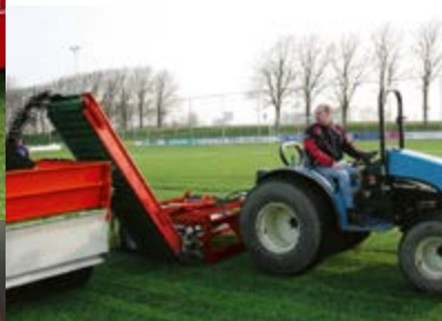
Easily adjustable rear roller controls working depth, whilst paddle brush extracts infill
