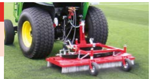
The 5 counter rotating brushes turn at high speed.
