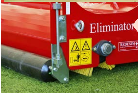
Easily adjustable rear roller controls working depth, whilst paddle brush extracts infill
