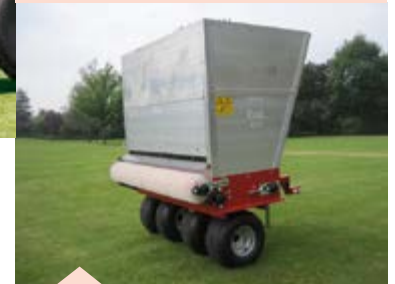
Options: A Hopper Extension kit increases the hopper capacity to 1.27m 3 .
