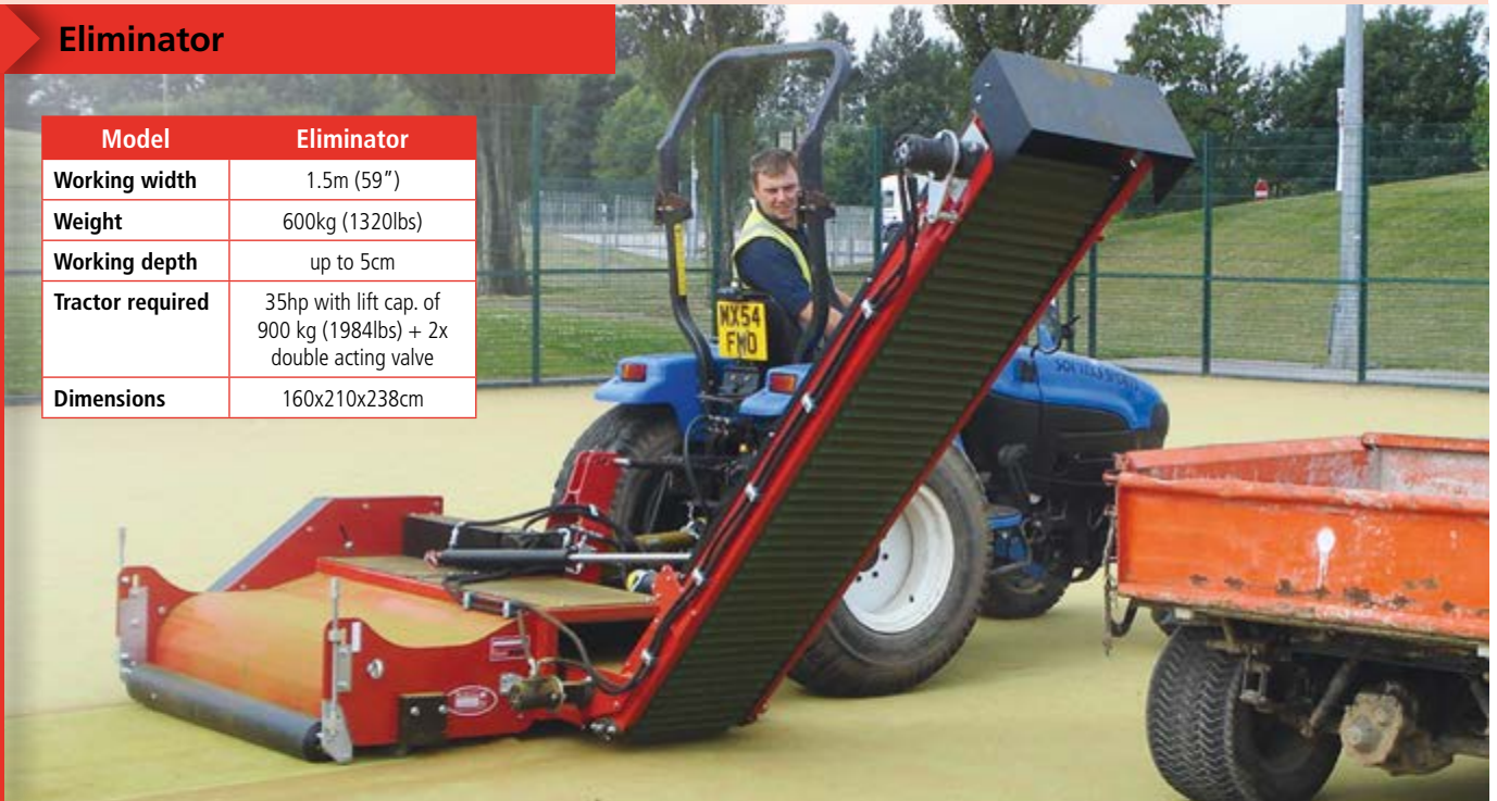
Easily adjustable rear roller controls working depth, whilst paddle brush extracts infill
