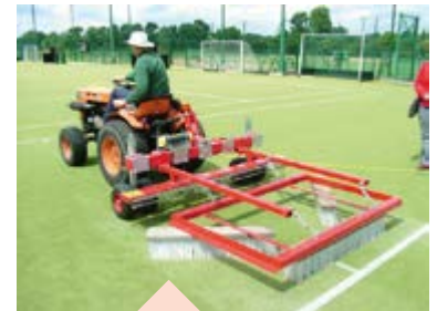
Optional-photo left: the mounting beam with rakes or pins can be exchanged for a beam containing a brush (L). Also a frame containing 3 brushes can be attached at the rear (R).
