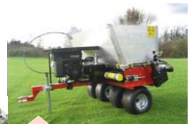
If a 13hp engine is added the Rink 1010 can be pulled by virtually any vehicle.
