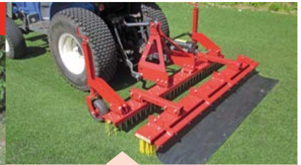
The Combi-Groom can be equipped with Ø5mm Rakes, and a magnet (photo under).
