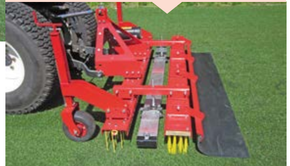
The Combi-Groom can be equipped with Ø5mm Rakes, and a magnet (photo under).
